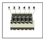
**PGED2** conducts I/O operations for the "Program Data" signal. Serial data for programming. **PGEC2** serves only as input for the "Program Clock" signal. Clock used for transferring the serial data (output from ICSP, input for the MCU).
