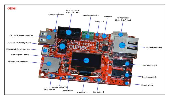
Hardware revision B of the board introduced a few changes to the layout:
