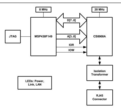
Figure 3. Hardware Block Diagram
