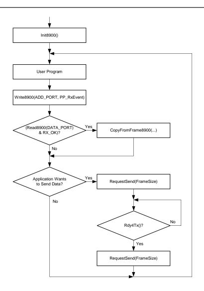
Figure 5. Using the Ethernet Module
