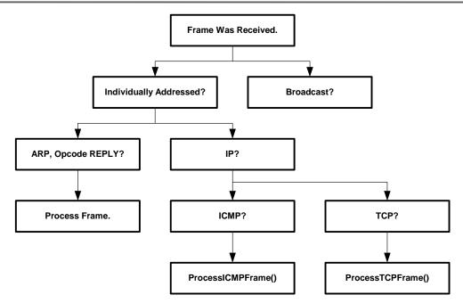
Figure 8. Demultiplexing of Received Frames
