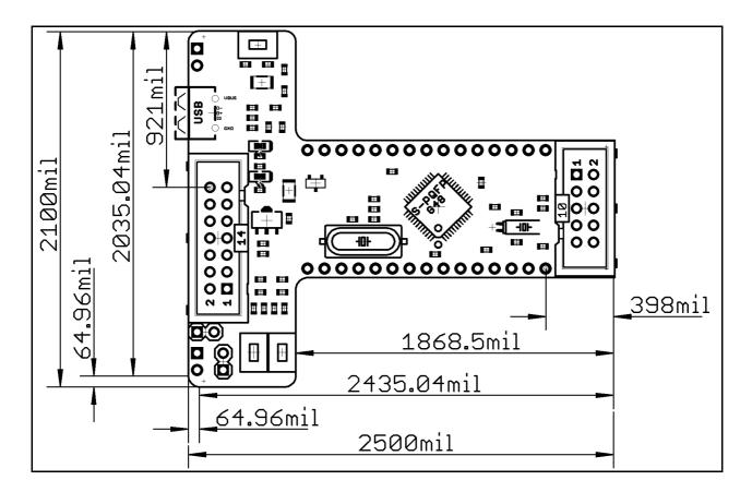
The highest elements on the board are the two connectors – UEXT and JTAG – 320mil each (without the PCB).
